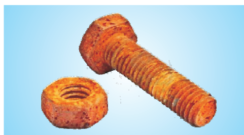
Fig. 4.9: Rusted nuts and bolts of iron
