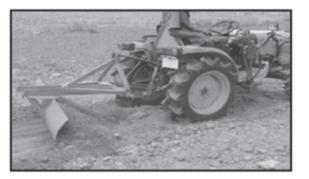
Fig. 15.5: Tractor drawn leveller
