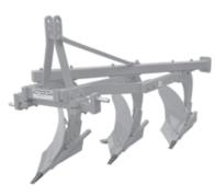
Fig. 15.1: Mouldboard plough
